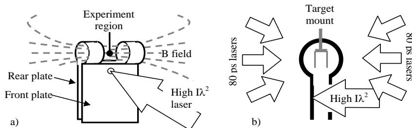
**FIGURE 4.** The mm-scale laser driven Helmholtz coil target. a) view of the laser entrance hole in the front and the loops, b) illustrates the multi-beam, target and diagnostic accessed required. In this view the 25 ps probe images the colliding plasmas in to the page. The loop radius is 1.25 mm, and the space between the inner edges of each loop is 2.5 mm. The foil targets are mounted across a 1.1 mm diameter hole on 2 mm wide, 10 mm long copper holders. The holders are separated by 1 mm.
