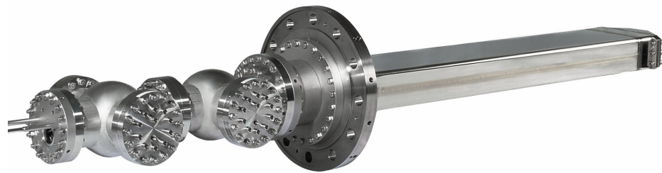
Figure 4.4: One of the two KB5 bolometer cameras
