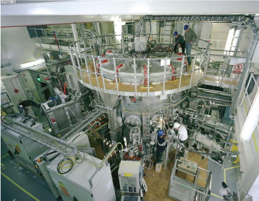
Figure 1.2: The MAST tokamak (the vessel has 4m diameter and 4.4m height)
