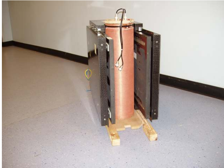
Figure 9.5: Laplacian's final magnet, ready for lab tests
