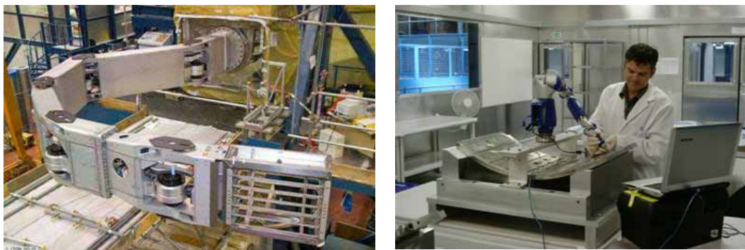
Figure 1.6: Left: The new lengthened Remote Handling boom during commissioning. Right: Inspection of the carriers for the Upper Dump Plate tiles in the Beryllium Inspection Facility
