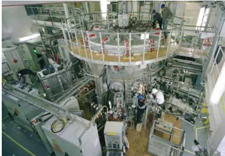
Figure 1.3: The MAST tokamak (the vessel has 4 m diameter and 4.4 m height)
