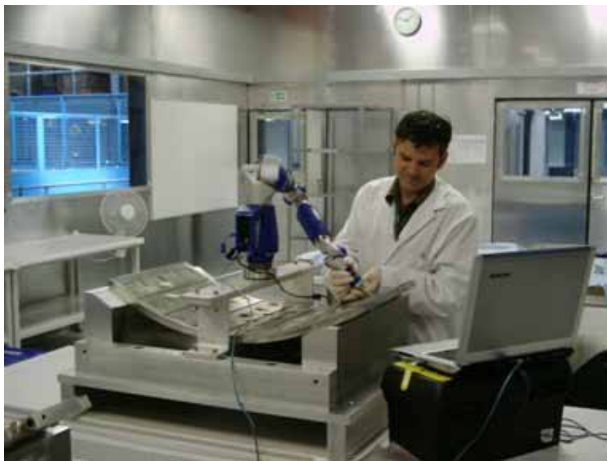
Figure 3.15: Inspection of the carriers for the Upper Dump Plate tiles in the Beryllium Inspection Facility
