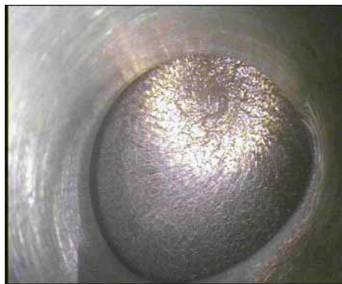
Figure 3.1: A close up view of the cooling channel of a neutral injection accelerator grid using an endoscope down the inlet water connection. Note the erosion pit in the copper material near the centre of the image caused by in the turbulent cooling water close to the inlet
