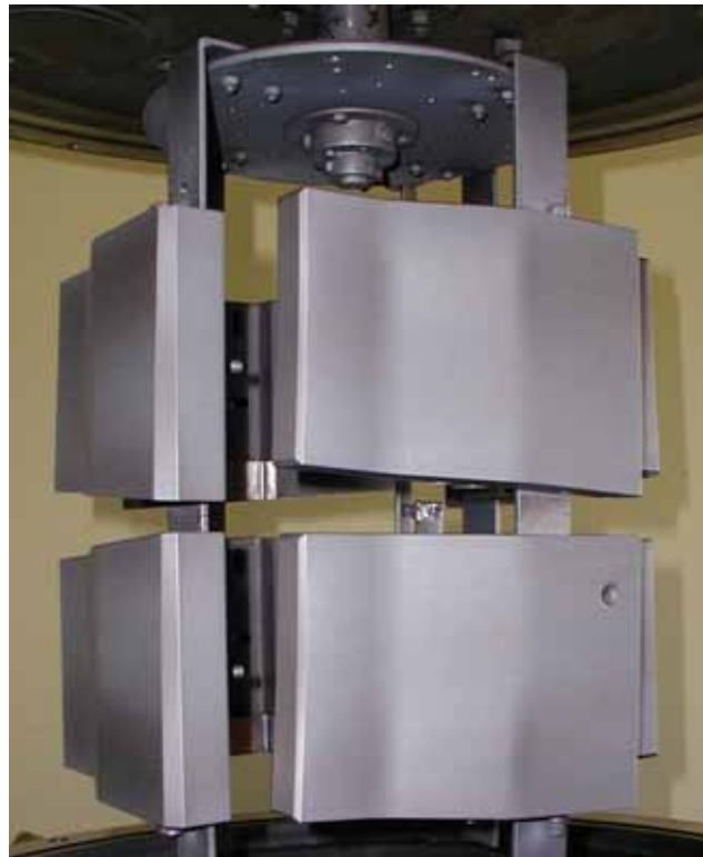
Figure 3.12: Tungsten coated JET divertor tiles during series production at MEdC
