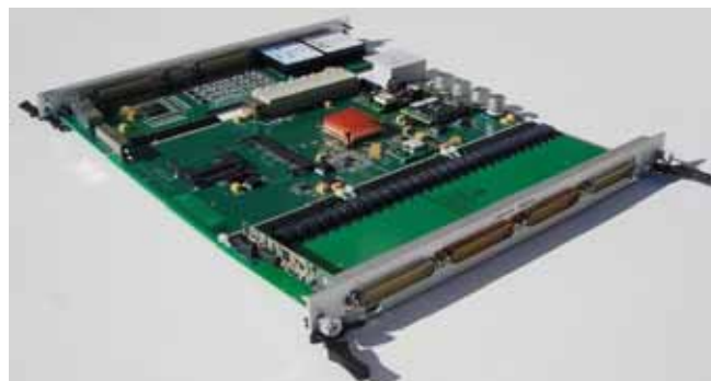
Figure 4.28: One of the new ATCA cards designed by IST (Portuguese Association) combining fast digitisers and FPGA-based processing to provide the ‘observers’ for the vertical position controller. Only one of the input digitiser cards is shown
