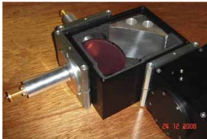
Figure 4.26: Two of the quasi-optical boxes for the new wideband reflectometer. The open box is fitted with two antennae and two waveguide transitions. A 60 GHz filter has also been inserted. these boxes serve as combiners, splitters and filters to allow the six microwave systems (four bands, all in X-mode and two of them also in O-mode), to use four waveguides to/from the torus
