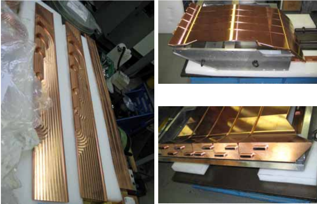
Figure 4.22: Components of the hypervapotron duct scrapers during manufacture and assembly
