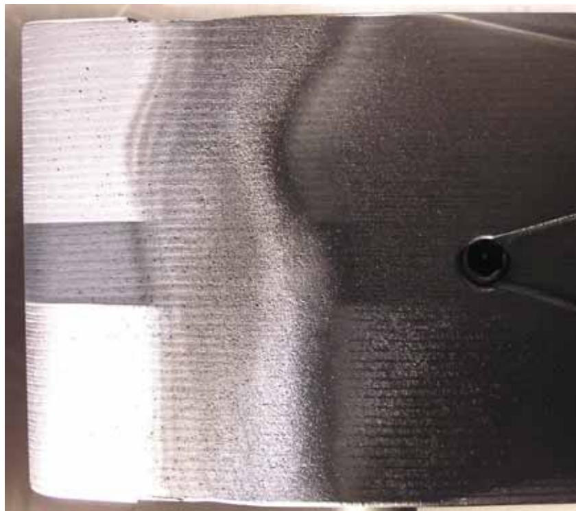
Figure 7.9: Photograph of tile 7X12L installed near the midplane of an Inner Wall Guard Limiter after exposure in JET 2004-07. Coatings of W and Re visible at the left of the tile have been totally eroded towards the right of the image
