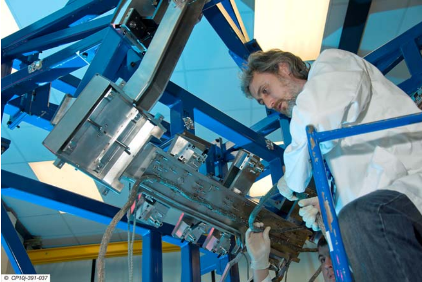
Figure 3.1: Trial assembly of diagnostic conduits on a full scale jig.
