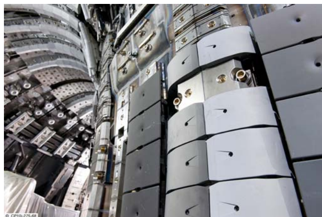
Figure 3.5: ILW tiles on the inner wall during Remote Handling phase 4.
