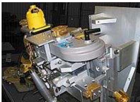
Figure 9.3: Bandsaw provided to JET by NIS Ltd.
