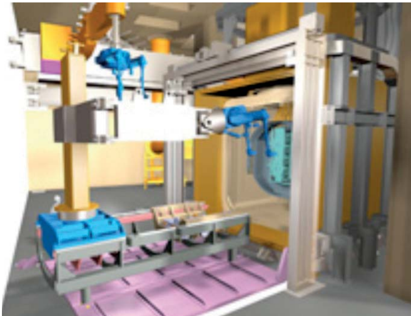
Figure 1.25: CCFE has an F4E grant to complete the conceptual design of the remote handling equipment of the Neutral Beam Cell in ITER. The image was generated during the Virtual Reality simulations used to validate the maintenance methodology of the accelerator source of the ITER NB heating system.
