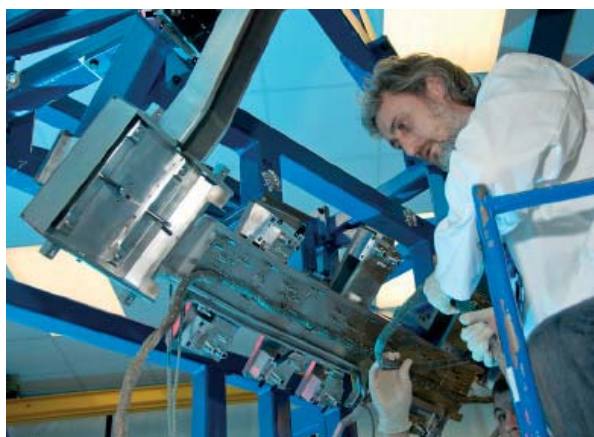
Figure 1.7: Trial assembly of diagnostic conduits on a full scale jig.
