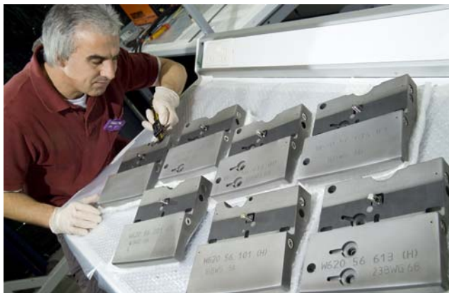
Figure 3.10: Assembly of metal parts into the back of tungsten coated carbon fibre composite tiles
