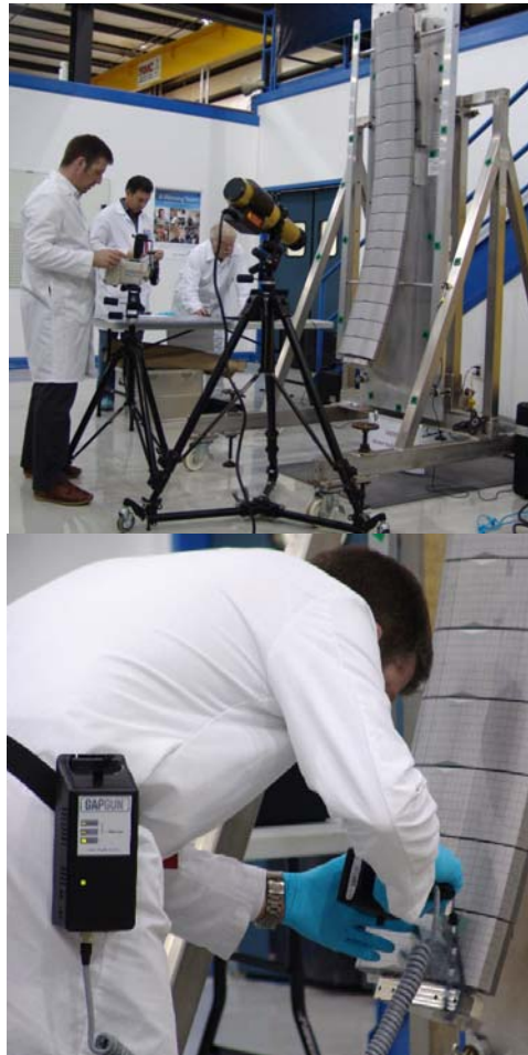
Figure 3.9: Assembly and inspection of the first 'Inner Wall Guard Limiter' on its jig at the beryllium manufacturer
