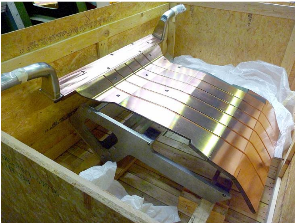
Figure 3.8: Photograph of new actively cooled neutral beam duct scraper panel
