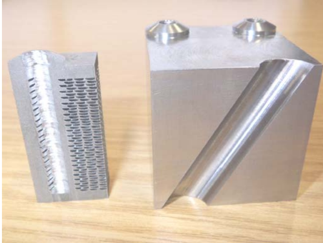
Figure 8.3: Diffusion-bonded test pieces
