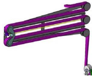
Fig 6 Upper Port Plug Cable management system
