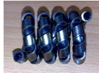
Fig. 3: Double spiral bimetallic spring
