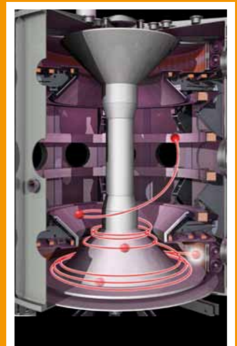
Detail of Super-X divertor showing particle exhaust path
