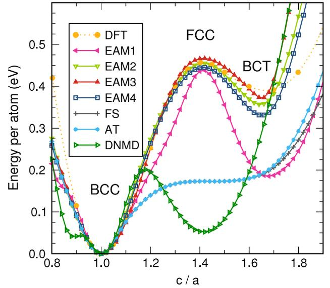
**Figure 3.** Variation of energy per atom calculated for the tetragonal Bain deformation pathway using the EAM potentials and DFT. The DFT PBE GGA data are taken from [13]. The reference energy is the cohesive energy of the BCC structure.
