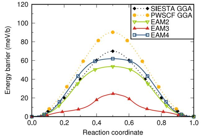
**Figure 6.** Peierls energy barrier calculated for tungsten using DFT and empirical potentials. The PWSCF and empirical potentials barriers were computed using the NEB method while the SIESTA barrier is computed using the reaction coordinate method.
