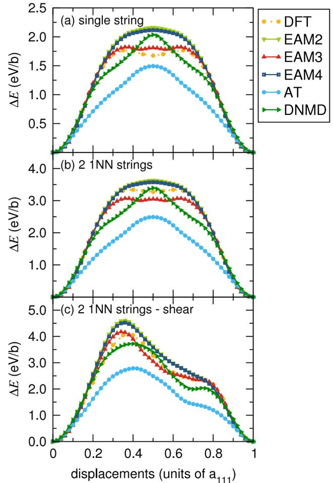
**Figure 4.** Energy variation associated with the rigid displacement of different strings of atoms: (a) a single [111] string displaced through the lattice; (b) two first-nearest-neighbour (two 1NN) strings displaced in the same direction; (c) two 1NN strings displaced in opposite directions (shear). The string displacement curves calculated using the empirical potentials are compared with those derived from DFT.
