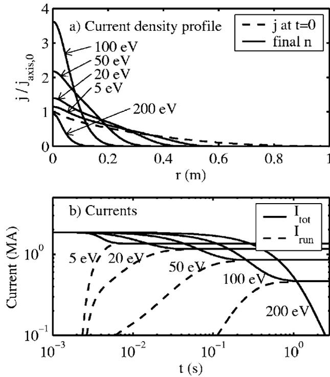
FIG. 5. For the five cases  $T_{\text{final}}=5$  eV ( $H=15$ ), 20 eV ( $H=11$ ), 50 eV ( $H=7.7$ ), 100 eV ( $H=4.0$ ), and 200 eV ( $H=-0.8$ ): (a) The final runaway current profiles and (b) the evolution of the runaway current and the total current.
