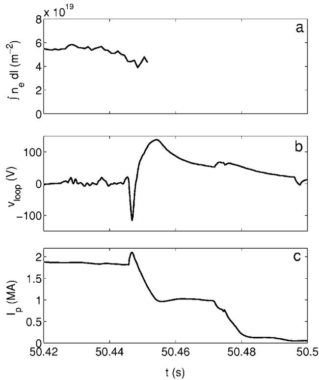
FIG. 1. Data from JET discharge 63 133 at the time of the disruption: (a) line-integrated density, (b) loop voltage at the vessel wall, (c) plasma current.
