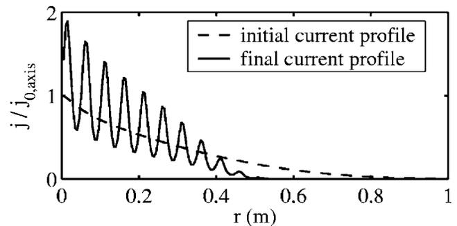
FIG. 9. The final current profile from a simulation where  $t_0$  has a 4% radial ripple.
