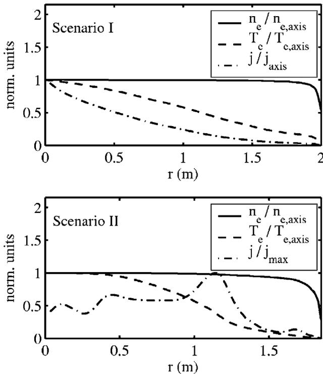
FIG. 10. Predisruption density, temperature, and current profiles for two different ITER scenarios.
