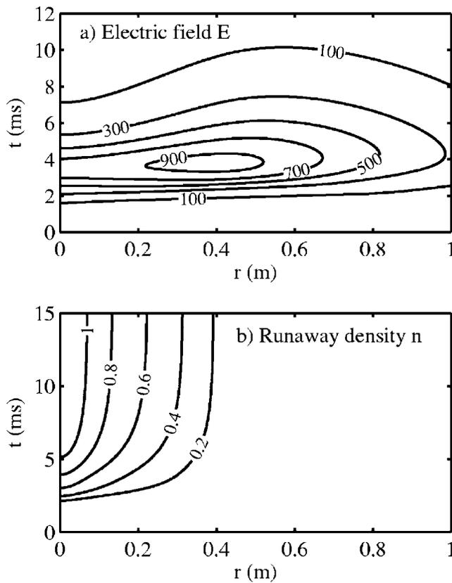
FIG. 3. Contour plots of (a) the normalized electric field and (b) the normalized runaway density from a simulation of the runaway dynamics in the disruption in JET discharge 63 133.
