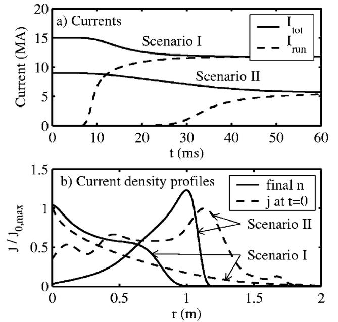
FIG. 11. Simulations of the runaway dynamics in ITER disruptions for scenarios I and II in Fig. 10.
