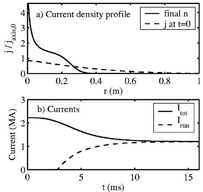
FIG. 8. An example of a more complex disruption scenario that can arise due to gas puffs or pellet injection. Here  $n_e$  rises to  $3n_{e0}$  and  $Z_{\text{eff}}$  increases from 1 to 1.5 during the thermal quench, and the onset is delayed 2 ms from the plasma boundary to the magnetic axis.
