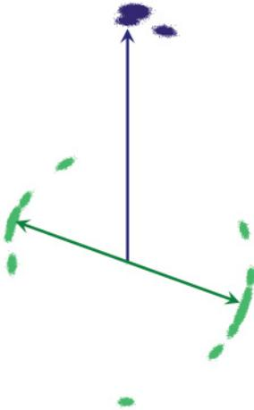
FIG. 7. (Color online) The MCE magnetic moments diagram for the (100) Fe/Cr interface. Fe moments are shown as dark-gray dots, Cr moments as green dots. Arrows represent directions of total magnetic moments for Fe and Cr subsystems.
