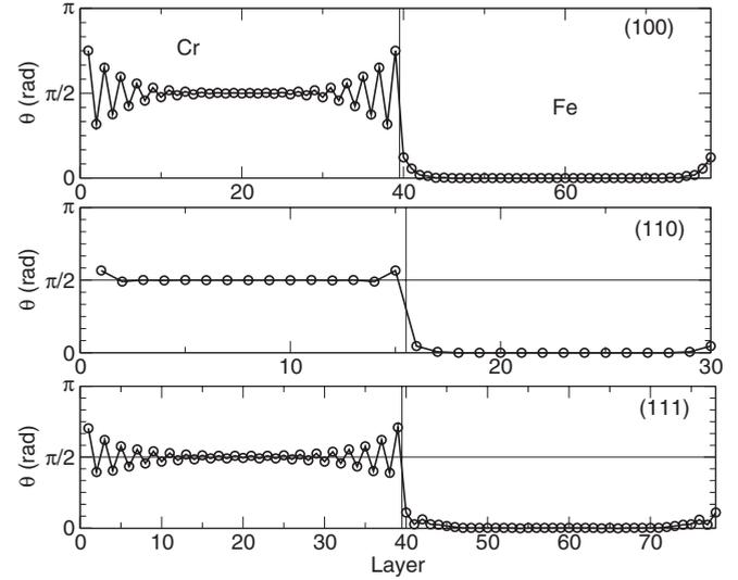
FIG. 5. Noncollinear DFT magnetic structures near Fe/Cr interfaces: absolute values of the angle between the local moments of various atoms and the moments of the inner bulklike Fe atoms. For the (110) interface, only the values corresponding to Cr atoms in one of the two columns in Fig. 1 are shown.
