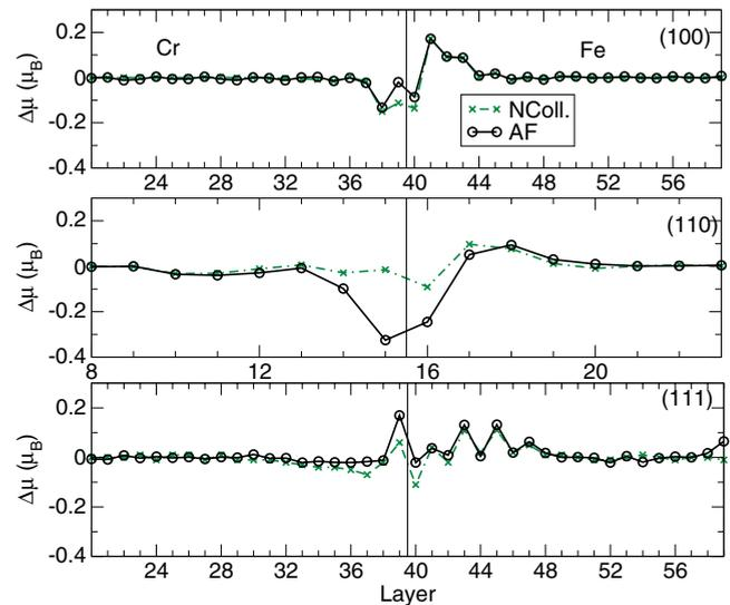
FIG. 4. (Color online) Variation of the magnitude of Cr and Fe DFT local moments (in  $\mu_B$ ) in the vicinity of the (100), (110), and (111) interfaces, in relation to their bulk values. Converged values are found for both collinear (Coll) and noncollinear (NColl) magnetic structures for the same supercells as those noted in Table I. For the (110) interfaces, only the values corresponding to Cr atoms situated in one of the two columns in the Fig. 1 are shown.
