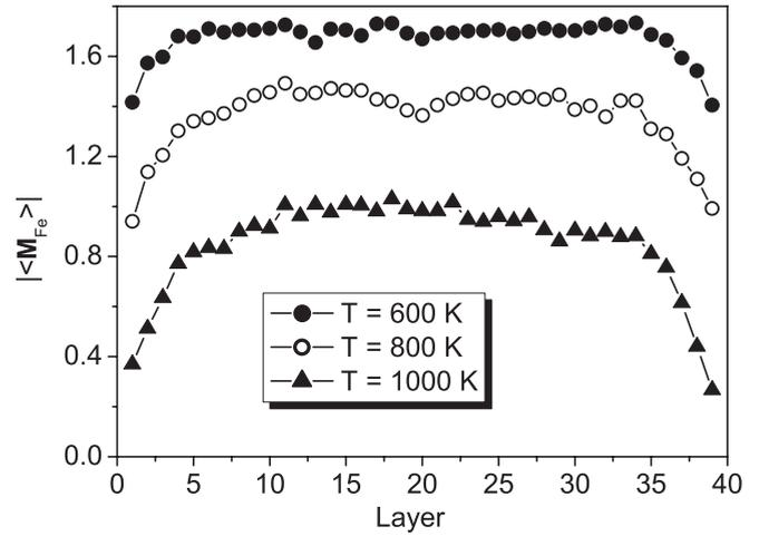
FIG. 11. Magnitude (in  $\mu_B$ ) of Fe magnetic moment vs atomic layer index at the (100) interface simulated using MCE for several temperatures.
