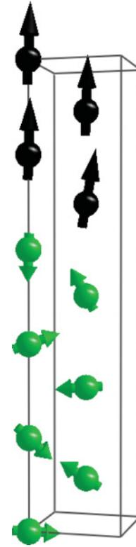
FIG. 6. (Color online) The MCE magnetic structure of the (100) Fe/Cr interface. Fe atoms are shown as black spheres, Cr atoms are green spheres.
