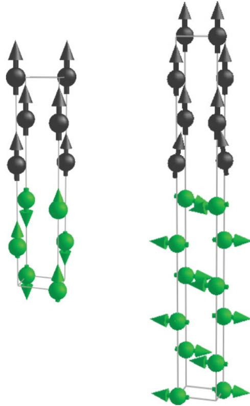
FIG. 1. (Color online) Schematic representation of the DFT magnetic structure of the (110) Fe/Cr interfaces with collinear (left) and noncollinear (right) magnetic order, showing Fe (black) and Cr (green) atoms near the interface. The magnitude and orientation of local magnetic moments are indicated by arrows.
