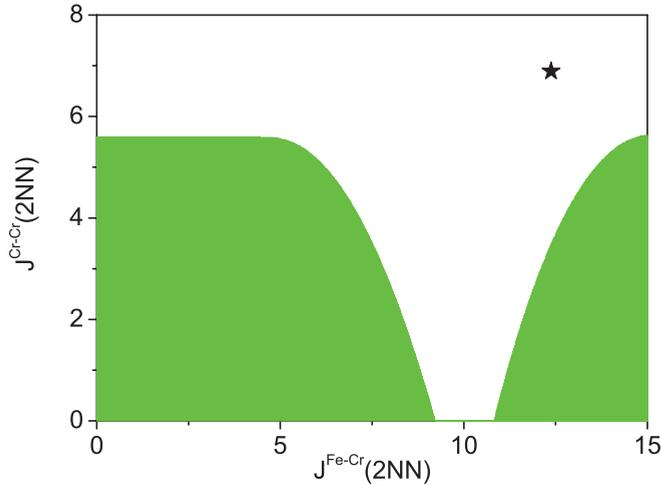
FIG. 13. (Color online) Regions in the space of the second-nearest-neighbor interaction parameters where the collinear magnetic structure at the (100) Fe/Cr interface is stable (shaded). The star sign indicates the actual values of these parameters in the MCE model.
