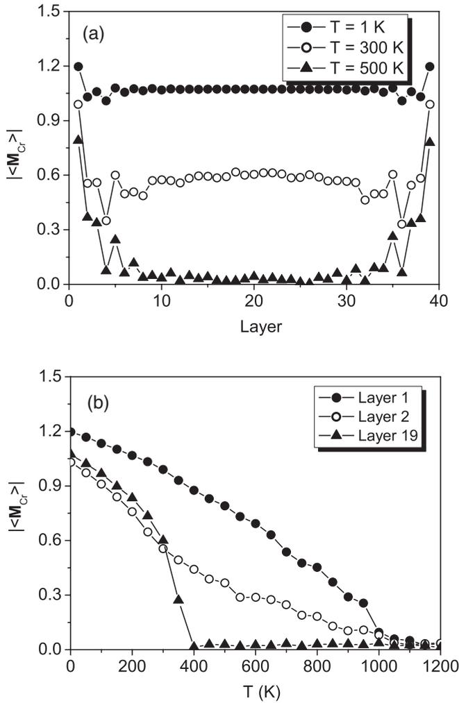
FIG. 10. Magnitude (in  $\mu_B$ ) of Cr magnetic moment shown as a function of atomic layer for the (100) Fe/Cr interface simulated using MCE for several temperatures (a), and the temperature dependence of the average MCE Cr magnetic moment near the Cr-Fe interface and in the bulk (b).
