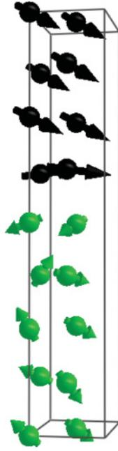
FIG. 9. (Color online) The MCE magnetic structure across the (110) Fe/Cr interface. Fe atoms are shown as black spheres, Cr atoms are green spheres.
