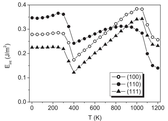
FIG. 12. Temperature dependence of the MCE interface formation energies.
