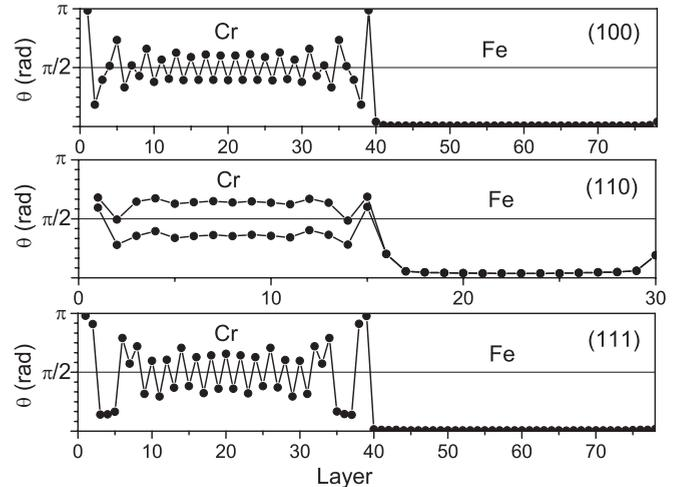
FIG. 8. Angle between the average Cr MCE magnetic moments in an atomic layer and the average Fe moment shown as a function of the number of the Cr layer. For the (110) Fe/Cr interface, two angles are shown for the Cr subsystem, corresponding to the two Cr columns with antiparallel (in the bulk) orientation of magnetic moments.
