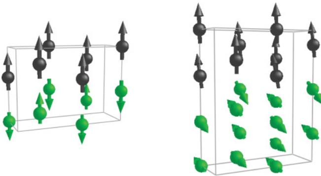
FIG. 3. (Color online) Schematic representation of the DFT magnetic structure of the (111) Fe/Cr interfaces with collinear (left) and noncollinear (right) magnetic order, showing Fe (black) and Cr (green) atoms near the interface. The magnitude and orientation of local magnetic moments are indicated by arrows.
