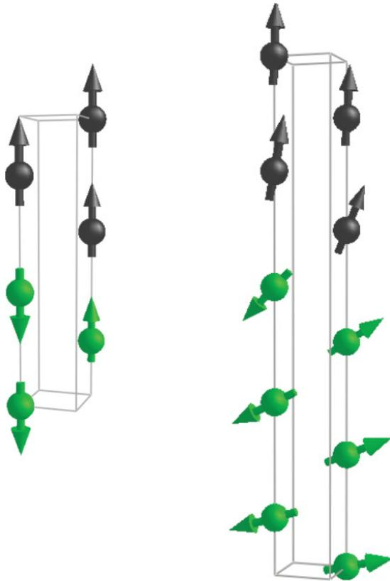
FIG. 2. (Color online) Schematic representation of the DFT magnetic structure of the (100) Fe/Cr interfaces with collinear (left) and noncollinear (right) magnetic order, showing Fe (black) and Cr (green) atoms near the interface. The magnitude and orientation of local magnetic moments are indicated by arrows.
