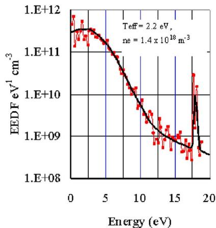
FIG. 1. EEDF measured with a 0.9-mm-diam spherical probe 17 mm in front of the plasma grid; arc power=45 kW, PG floating, 0.3 Pa, H<sub>2</sub>.
