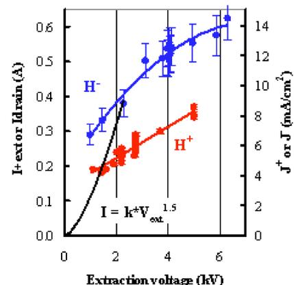
FIG. 6. Positive and negative ion currents ( $I_{ext}^+$  and  $I_{drain}$ ) and current densities ( $J^+$  and  $J^-$ ) extracted from the Kamaboko III source vs the extraction voltage. The negative ion data have been corrected for drift (in time) due to tungsten contamination of the plasma grid surface. The H<sup>+</sup> data were taken with an arc power of 45 kW, the H<sup>-</sup> data with 20 kW, both with 0.3 Pa, H<sub>2</sub>.
