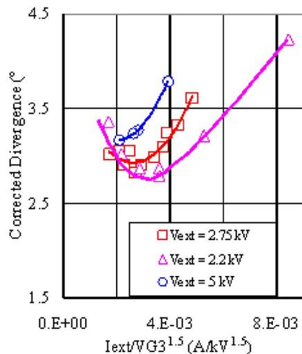
FIG. 4. Beamlet divergence measured in the horizontal direction as a function of the perveance for different values of the extraction voltage. Arc power=20 kW, 0.3 Pa, H<sub>2</sub>.
